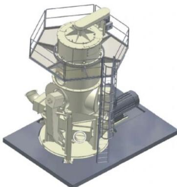
In general, coal pulverisers are designed to achieve the maximum rated capacity grinding a design coal with a grindability of 55 HGI and 8-12 per cent moisture and achieving a discharge fineness of 70 per cent passing a 200 mesh screen (74 micron) and 99.5 per cent passing a 50 mesh screen. Variation of the coal hardness and/or moisture content will effect, up or
