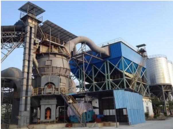
**Equipment Type:** GRMS46.41 Slag Vertical Roller Mill
