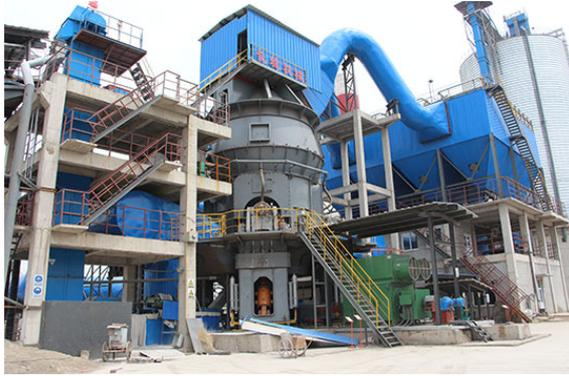
**Equipment Type:** GRMS46.41 Slag Vertical Roller Mill
