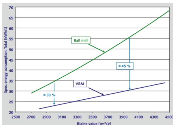
Traditionally, the closed circuit ball mill with high efficiency separator has been the most common system for cement grinding. However, as happened with raw grinding over the last 25 years, the vertical roller mill (VRM) is now successfully being used for many clinker grinding applications and is rapidly becoming the standard for new grinding installations. The first such [vertical roller mill](#) installation in the United States was
