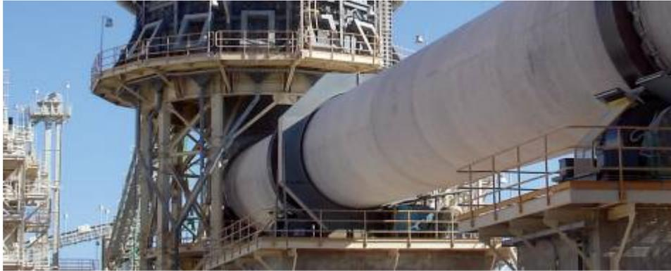
That is accomplished by skewing the roller shafts at slight angles to the rotary kiln shell and it is also known as training the kiln.
