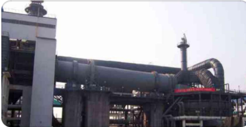
The [rotary kiln](#) is a refractory lined cylinder rotating about its axis. The rotary kiln slopes slightly downward from feed to discharge end. The slope and rotation of the kiln move the material through it. Rotary Kiln speed is variable to vary pellet retention time. The rotary kiln is a single chamber with an open feed end connected by housing to the grates preheat furnace.
